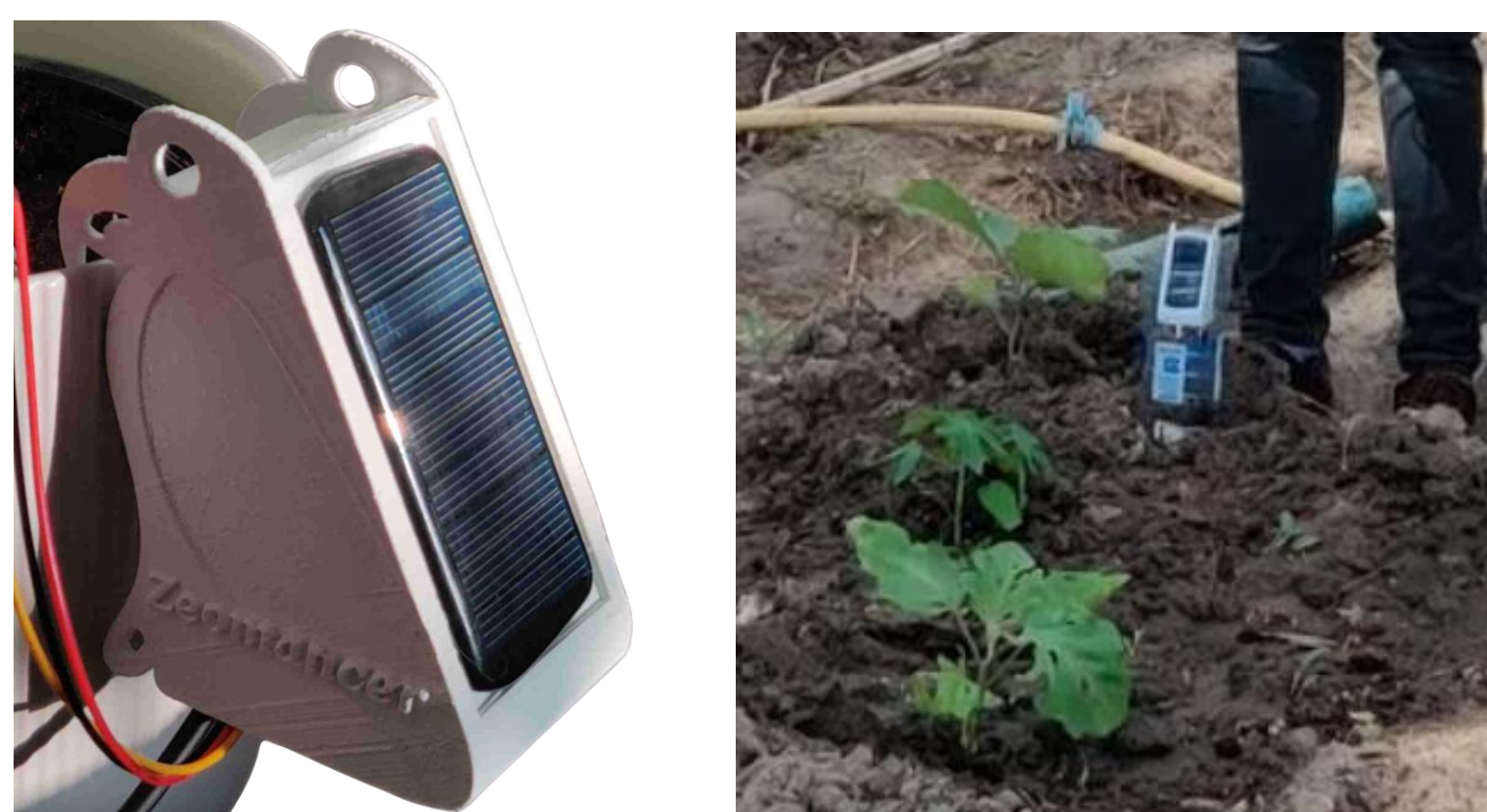
Figure 1. First Zeomancer prototype deployed at the University of Dar es Salaam demo farm with Dr. Moses Ismail and two crop scientists. This device also has a soil moisture sensor installed and is mounted on a water bottle. Photo: Brian Rowe.
